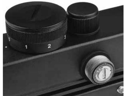
Once the protective black caps have been removed, you can adjust the elevation and windage. Insert either a coin or small flat-bladed screwdriver into the slot on top of the knob and turn. You will hear and feel noticeable clicks to make it easier to adjust and readjust your dot sight.
