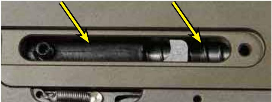
Using a high-quality gun lube (do not use household oil such as WD-40 or silicone), put 2-5 drops on the two bolt sections shown above. Drop the lube along both sections. Replace the transparent faceplate.
