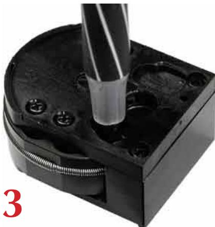
Image 3: Press the tip of a ballpoint pen into pellet's skirt to properly seat it.
