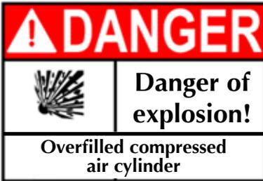
**Do NOT exceed maximum fill pressure of 200 bar at room temperature!**
