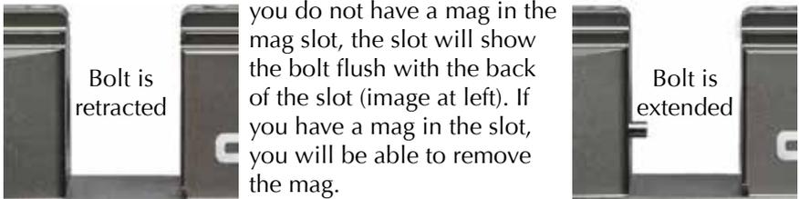
If you cannot insert/remove a mag, the bolt needs to be retracted:
