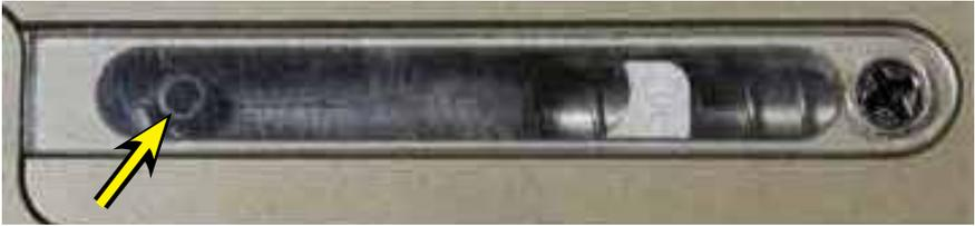
On the right side of the receiver, you will see the above window. The Allen screw (arrow) indicates the correct position when the bolt is retracted. If
