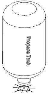
**( Important!! Apply vertical force onto tank only or the fill stem will be broken.)**
