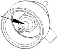
Apply some silicon oil onto on Parts #3 (internal stem) in order to make the installation easily. There is an o-ring inside the head of propane tank. Make sure the o-ring is not defective. If the o-ring is crushed, the internal stem will have great friction during the installation.
