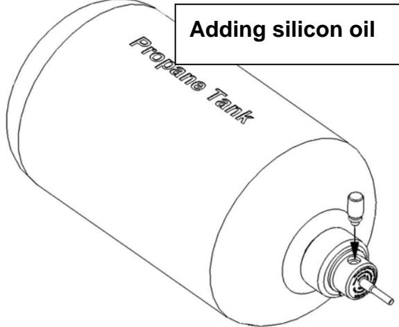
Take off Parts #8 (Silicon oil adapter) and drop some silicon oil in order to lubricate your GBB Airsoft. Then, put part #8 back to XG02. (Propane gas is dry and doesn't come with oil.)NOTE: \* If there is propane leaking when you take off #8 silicon oil adapter, please uninstall XG02 immediately. You either don't install XG02 correctly or your XG-02 is not working functionally. \*\* When you put part#8 back to XG02, please remember the oring (parts #10) is still there.
