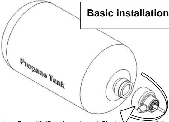
Smoothly turn Parts #6 (Rotating adapter) Clockwise to install the XG-02 adapter. Do NOT cross the adapter threads! If there is any leaking after you install the XG-02, please take XG-02 out of propane immediately. Leaking only happens when you didn't install correctly. (\* How to tell it is leaking? You can hear the leaking sound and you can smell the propane odd odor.) (\*\* When you take off XG02 from Propane tank, remember to hold tight of both XG02 and tank.)
