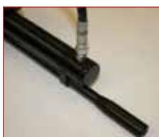
**To fill the Leopard air rifle:** Attach the stainless steel fill adapter to the correct fill equipment. Rotate the fill port's protective cover to allow access. Insert the fill adapter into the fill port.
