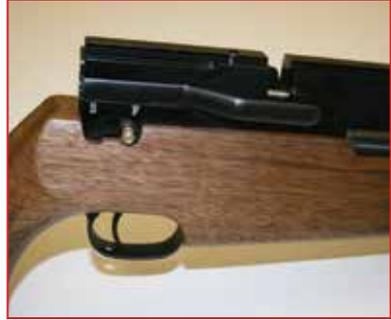
In addition to the safety catch, a loaded and cocked rifle can be made safe by decocking (uncocking). To decock the rifle, first pull the sidelever back to the rear position and remove the magazine. While holding the sidelever, squeeze the trigger and let the lever return forward under your control. The rifle is now decocked.
