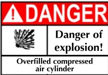
When filling the compressed air cylinder, the compressed air must NOT contain oil, water or any other contaminant.
