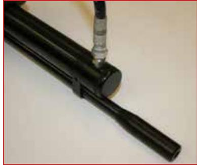
2) When charging is complete, bleed the excess air using the fill apparatus bleed screw and remove the fill adapter from the rifle. When finished, rotate the protective cover to prevent contamination of the fill port.
