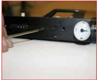
**NOTE:** This adjustment affects sear engagement. It may be necessary to alter both adjustments to achieve the desired setting. Adjustment of one screw may affect other settings. **Do not over-adjust, as this may cause the gun to fire prematurely or not operate correctly and make the rifle unsafe.** Always check your settings to ensure correct and safe operation of the rifle. Always ensure that operation of the safety is unaffected by any alterations you may make to the trigger mechanism.
