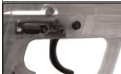
Fig. 2B - Push rearward for "OFF SAFE"
