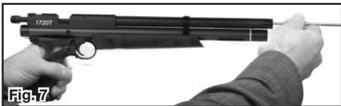
**Note:** The bolt must be cocked and open for the jammed pellet to clear the breech when it is pushed out by the ram rod.
