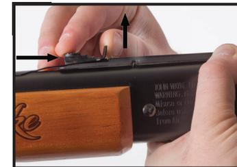
7) Insert the two (2) black nylon spacers between the mount and the receiver. Align the spacers under the rear anchor hole in the mount and over the stock screw hole.
