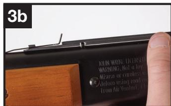
4) Align the rear anchor hole in the mount over the hole for the stock screw at the top rear of the receiver.
