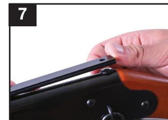
8) With the front of the mount secure and the spacers installed, place the lock washer on the rear stock screw. Replace the stock screw using a phillips head screwdriver by turning clockwise.
