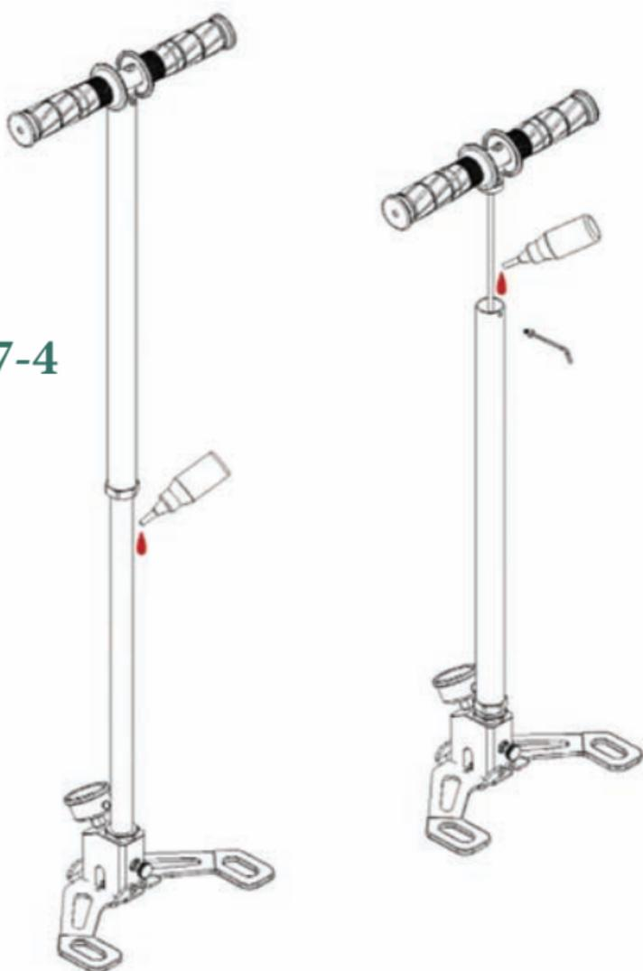
Lubricate pump with silicone oil as shown.
