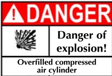
Do **NOT** exceed maximum fill pressure of **310 bar/4,500 psi** at room temperature!
