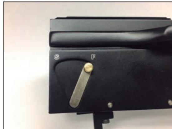
In addition to the safety catch, a loaded and cocked rifle can be made safe by decocking (uncocking). To decock the rifle, first pull the sidelever back to the rear position and remove the magazine. While holding the sidelever, squeeze the trigger and let the lever return forward under your control. The rifle is now decocked.
