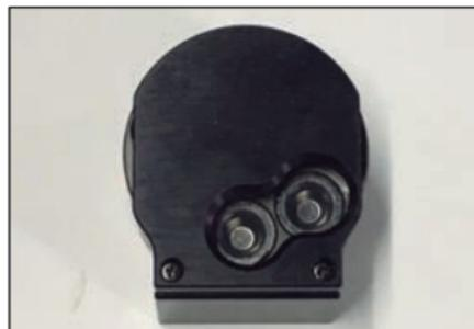
After seating pellet, turn mag to expose the next open hole and seat your next pellet or bullet. Repeat steps 1-5 until mag filled.
