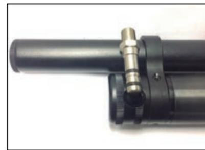
Do not use any other type of adapter other than the one supplied with the rifle. Slowly fill the rifle to a MAXIMUM of 230 bar (approximately 3,330 psi) pressure. Filling the rifle too fast is unsafe and creates excess heat that may result in a low or inaccurate fill pressure. Do not overfill as this will damage the gun and result in low power. Such damage is not covered under warranty.
