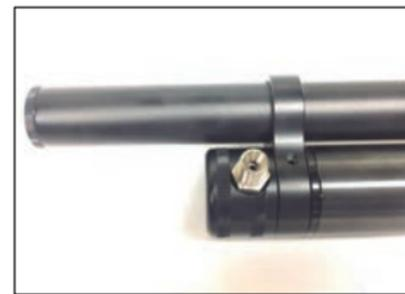
When charging is complete, bleed the excess air using the fill apparatus bleed screw and remove the fill adapter from the rifle.
