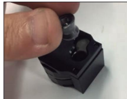
Insert a pellet into the hole on the lower left
