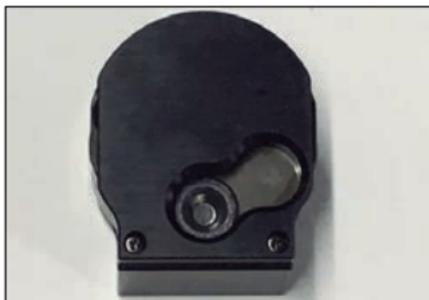
First pellets has been inserted & properly seated.
