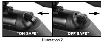
**⚠ ATTENTION:** BEFORE YOU PUT YOUR AIR RIFLE "OFF SAFE", BE ABSOLUTELY CERTAIN THAT YOUR AIR RIFLE IS POINTED IN A SAFE DIRECTION AND THAT YOU ARE READY TO FIRE. ONCE YOUR AIR RIFLE IS COCKED AND AUTOMATICALLY "ON SAFE", DO NOT RECOCK THE AIR RIFLE WHILE IT IS LOADED TO PUT IT BACK "ON SAFE". SEE "STEP 1. OPERATING THE SAFETY" FOR INSTRUCTION ON HOW TO PUT THE TALON MAGNUM AND FALCON HUNTER BACK "ON SAFE".
