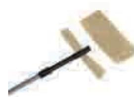
Cut the cloth or paper towel in the size as shown above. Fold the material to fit through the loop. Adjust the length of the material to smoothly enter the barrel. otherwise too much material will get jammed in the inner barrel and can cause the hop up bucking to get out of place.
