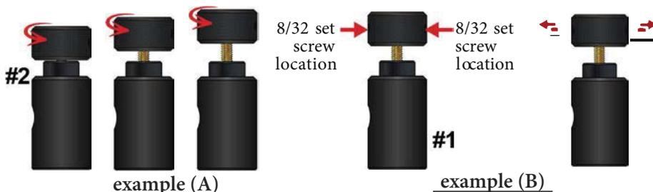
3: To remove the UFA knob, ensure the 8/32 set screws are loosened and turn the UFA knob (**part 2**) counter clockwise towards the “closed” position until the UFA knob is fully removed from the UFA pin as shown in **example: (C)**.
