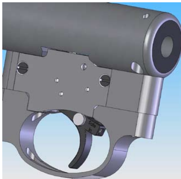
With the button out the rifle is now ready to fire.
