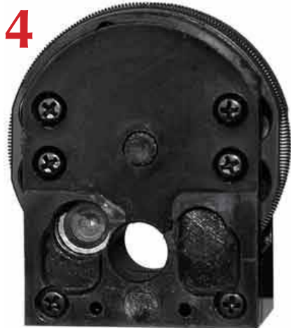
Image 4: First pellet has been inserted & properly seated.
