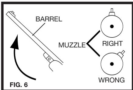
front sight is pointed upward, because the gun will not feed properly if it is on its side. (Fig. 6) The BB can be seen on the magnetic tip (after the bolt handle is released) by looking into the feed track. If a BB did not feed onto the magnetic tip, shake the gun slightly and repeat the "LOADING BBs" instructions.
