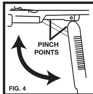
**CAUTION:** Be sure to grasp forearm firmly as you close the lever to prevent it from snapping back and causing possible injury. Also, be careful to keep fingers out of cocking mechanism when closing lever (See "PINCH POINTS", Fig. 4). Never put your finger on the trigger until you are ready to fire.
