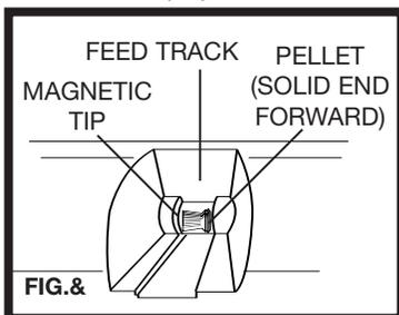
**LOADING PELLETS:** With BBs removed from the magazine (See "EMPTY BB MAGAZINE, Page 5), lower muzzle slightly and pull bolt handle rearward. Then place a pellet (solid end forward) in feed track. (Fig. 7)
