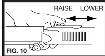
The Model 840/841 is equipped with a rear sight that is adjustable for elevation. Raise the rear sight to make the gun shoot higher. Lower the rear sight to make the gun shoot lower. (Fig. 9 & 10)
